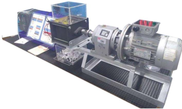
*Figure 1. Container grinding system.*
