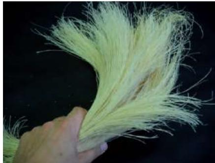
*Figure 1. Bamboo technical fibres after mechanical extraction*
