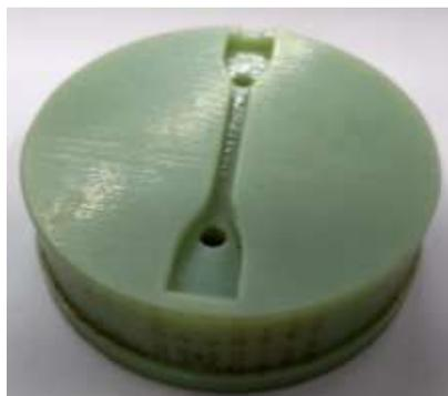
Figure 3: Insert made with polyjet technology. GITEM UAO Research group
