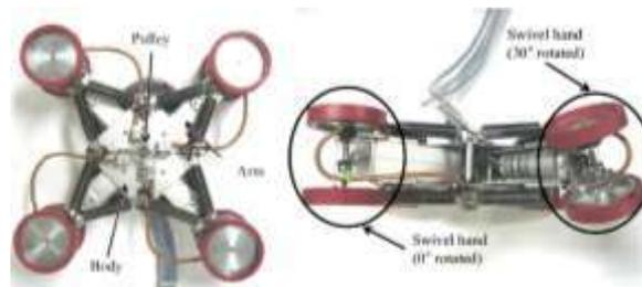
Figura 3. The prototype of the in-pipe robot [6].
